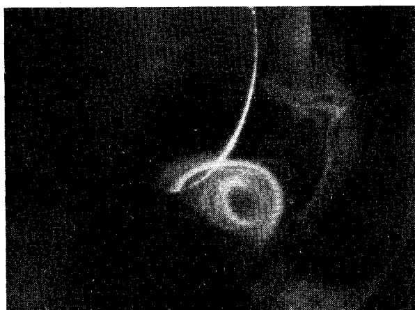
Fig. 9 Early stages of vortex roll-up on source side of 25.4 mm orifice ( f=40 Hz).
